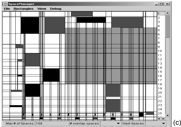
Figure 13: Space manager applied to automated information visualization system. (a) Folders on timeline contain data about patient's operation. (b) Visualization system uses space manager to position and scale selected folder to reach largest size possible at its original aspect ratio without overlapping important objects. (c) Space manager debugging tool shows dark full-space rectangles and edges bounding empty spaces used to calculate enlarged folder. Gridded timeline background and selected folder in (a–b) are deleted from spatial representation by visualization system to allow scaled folder to overlap them. Large light gray rectangle at right is largest empty-space rectangle selected by query to contain scaled folder. (d) Pseudocode for query that selects largest empty space. Allocation strategy must also determine where to place object in selected largest empty-space rectangle.
