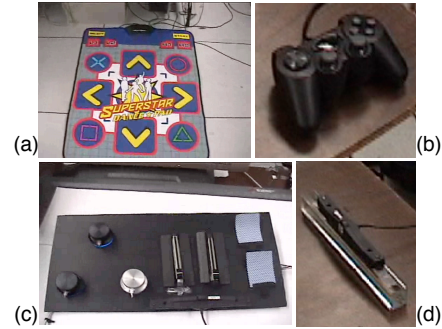
Figure 3. Input devices used in our prototype: (a) Dance mat. (b) Game controller. (c) Tracked board with PowerMate sensors (left) and MIDI sensors (right): sliders and bend sensors attached to playing cards. (d) Wand with attached InterSense 6DOF tracker.
