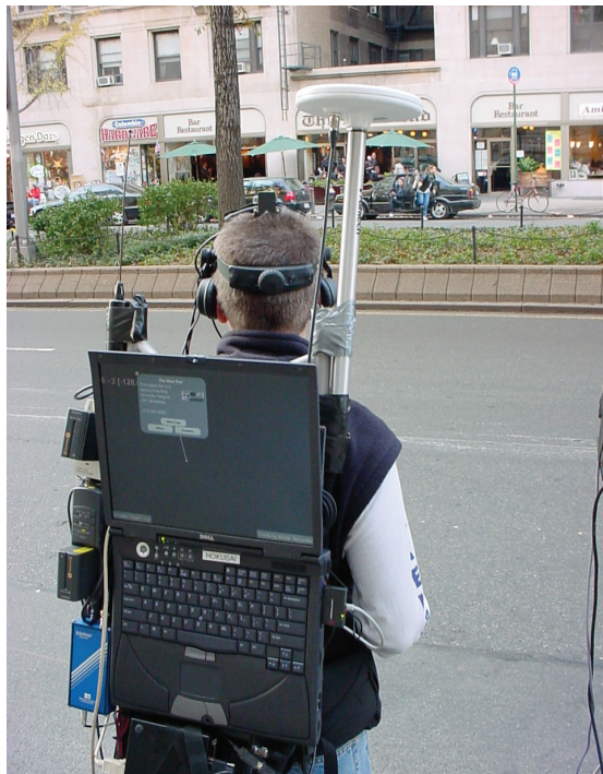
5 Outdoor mobile AR system presents overlaid graphics on a tracked see-through head-worn display.
