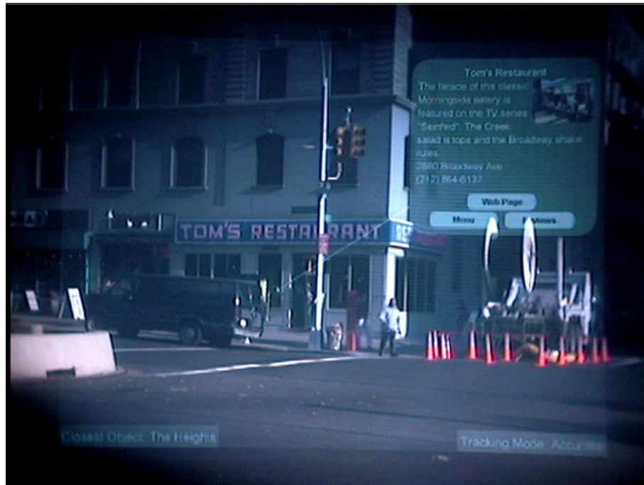
Figure 3.17 Image taken directly through an optical see-through head-worn display of restaurant and related popup information
