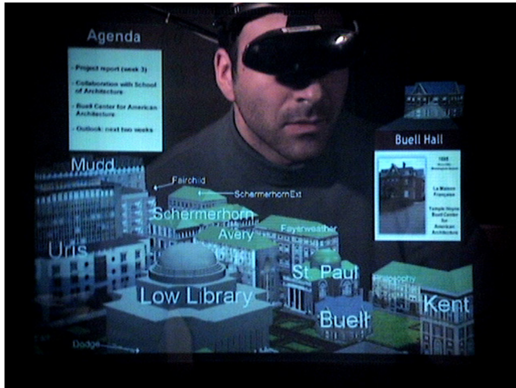
Figure 1.2 View management in an augmented reality meeting scenario (imaged through a tracked, optical see-through, head-worn display).
