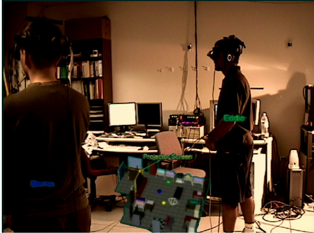
Figure 3.31 A notification rule that points out (imaged through a tracked video see-through display) any display that two users are viewing and is not in the local user's field of view. In this case, the Projection Screen fits the rule, resulting in the display of a related label in the aid.
